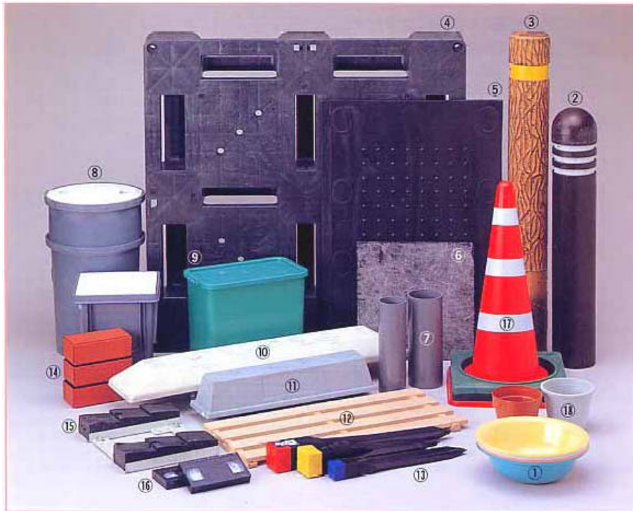
Figure 3 Examples of recycled plastic products through material recycling
